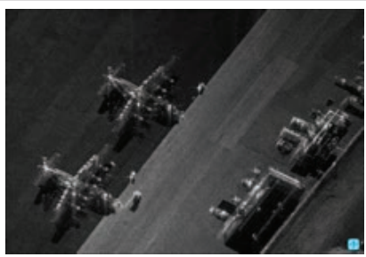
SAR Image of C-130 Aircraft on Flight Line at Kirtland AFB, NM Courtesy of Sandia National Laboratories, Radar ISR'
